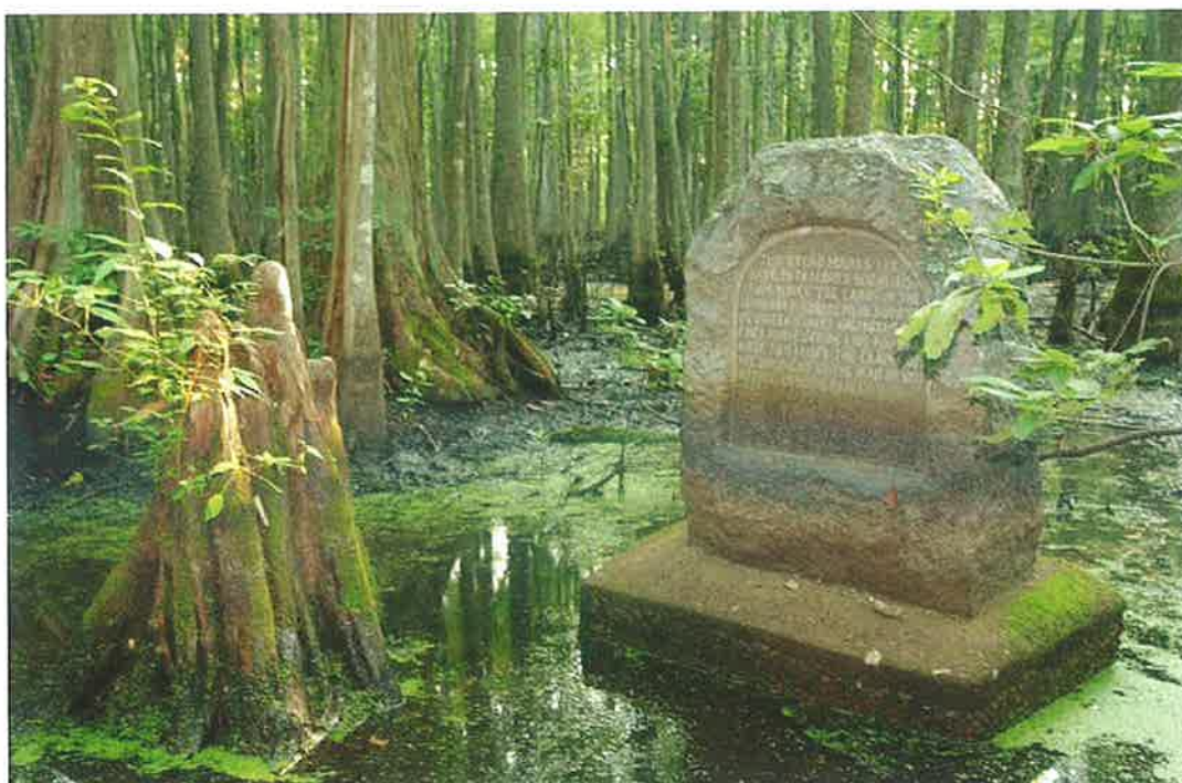
FIGURE 3 Monument marking the Initial Point of the 5th Principal Meridian (Photo provided by the Arkansas Society of Professional Surveyors)
